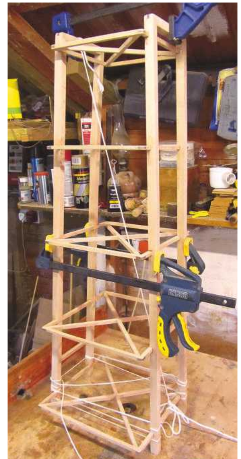
▲ Pic 6. Getting all the joints up tight with the shelves level required, as always, several clamps. In this project, it also required diagonal bracing with string
